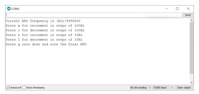
Follow the instructions till you get the right BFO frequency for your set. You may use any Audio spectrum analyzer to ensure the pass band noise of the set is within 300Hz to 3200Hz.
