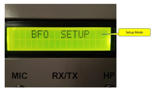
The set is now operating with last tunned VFO and current BFO value and the Serial monitor of Arduino IDE with show below setup screen.
