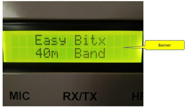
After the banner has been displayed, the set will go into operation mode with initial frequency of 7050 Mhz as displayed on the LCD screen below.
