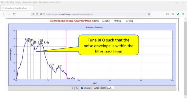
Tune the BFO such that the max audio amplitude falls within 300Hz – 3200Hz filter band width.
