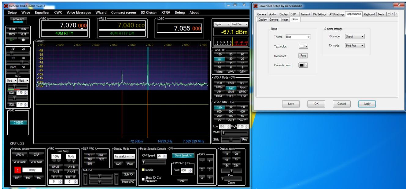
To change the way the signal looks on panadapter you can adjust display grid Max level and Low Level. Low level should be set close to your noise floor. That way the waterfall won't be all red with the noise.
