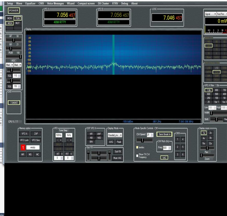
First thing we are going to do is adjust the trimmers, R9 and R10 back and forth until we get the LO(2) reduced as far as we can go while transmitting into a dummy load. Make sure you monitor the PA heat sink! Let cool between adjustments as necessary!
